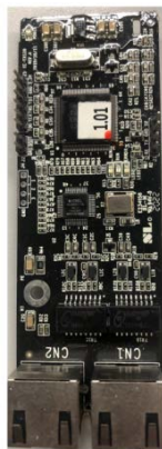
EtherNet IP/Modbus TCP EC-TX510/515
